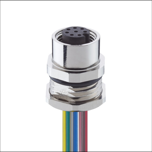
M12 panel mount connector, female, A-coded, IP67, for front mounting, thread M16, with nut and stranded wires
